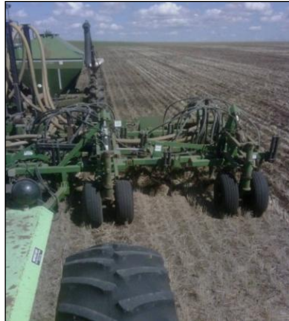
Photo 1. Our 4WD tractor and air drill are modified to travel on permanent tram lines. Source: S. Larocque
