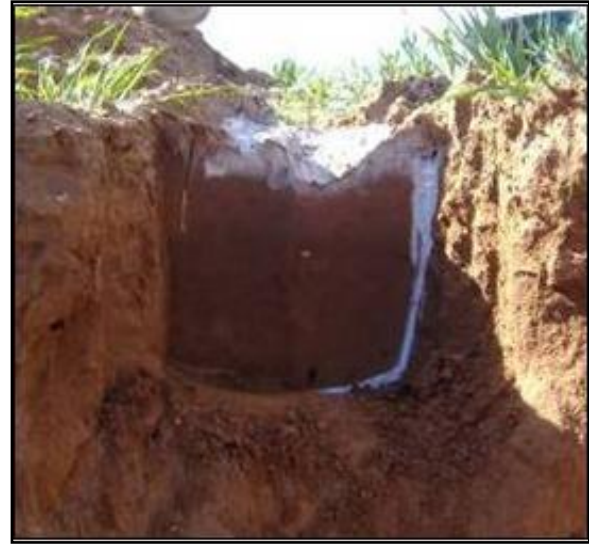
Photo 8 (left). Latex paint on untracked area. Photo 9 (right). Latex paint on tracked area, after one pass of a field sprayer. Source: R. Ruwoldt
