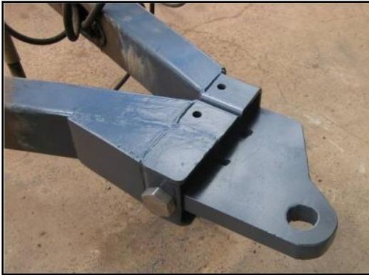
Photo 20 (left). 7.5-inch offset drill hitch. Source: S. Larocque. Photo 21 (right). 6-inch offset air tank hitch. Source: S. Larocque
