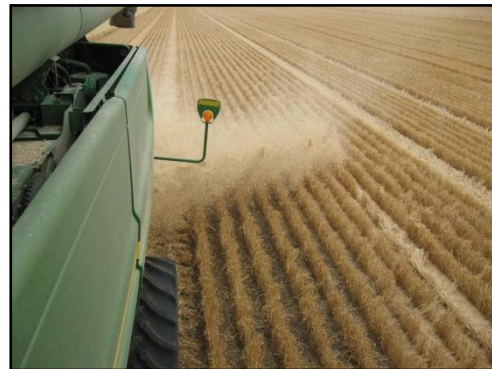
Photo 14. Spreading chaff across the entire width of the header is important. Source: R. Ruwoldt
