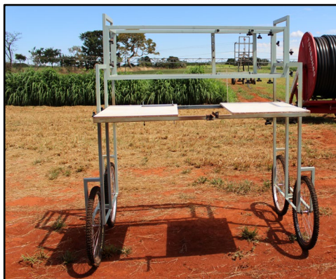
Figure 3. Research cart for carrying thermal, fluorescent and multispectral sensors at Embrapa Cerrados, Brazil (Source: Author).
