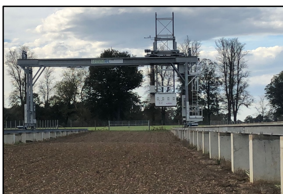
Figure 4. A) Field Scanner at Rothamsted Research Farm, United Kingdom (UK) contains numerous proximal sensors that can be positioned over crops within a 10m x 120m area (Source: Author, 2018). B) The Field Scanner is comprised of a chlorophyll fluorescence sensor, NDVI sensors, two hyperspectral imagers, twin scanning lasers for 3D visualization, carbon dioxide sensor, thermal infrared camera and red-green-blue (RGB) camera. The platform of sensors allows for automated 24 hour monitoring of crops throughout the season to observe crop architecture, crop health and crop development (Source: Author, 2018).
