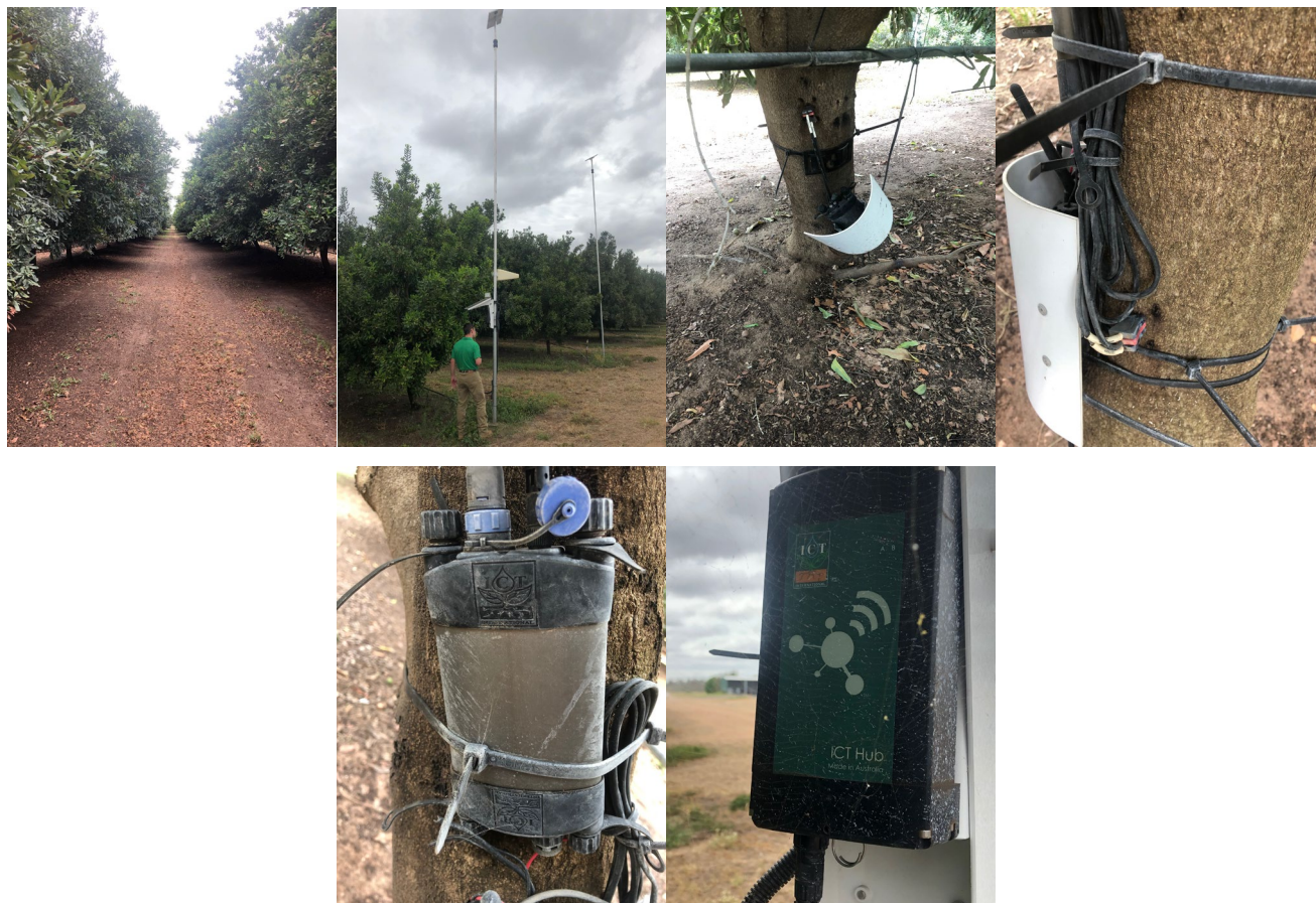
Figure 15. Telemetry on proximal sap and water flow sensors on Macadamia Trees, QLD, AUS (Source: Author, 2019).
