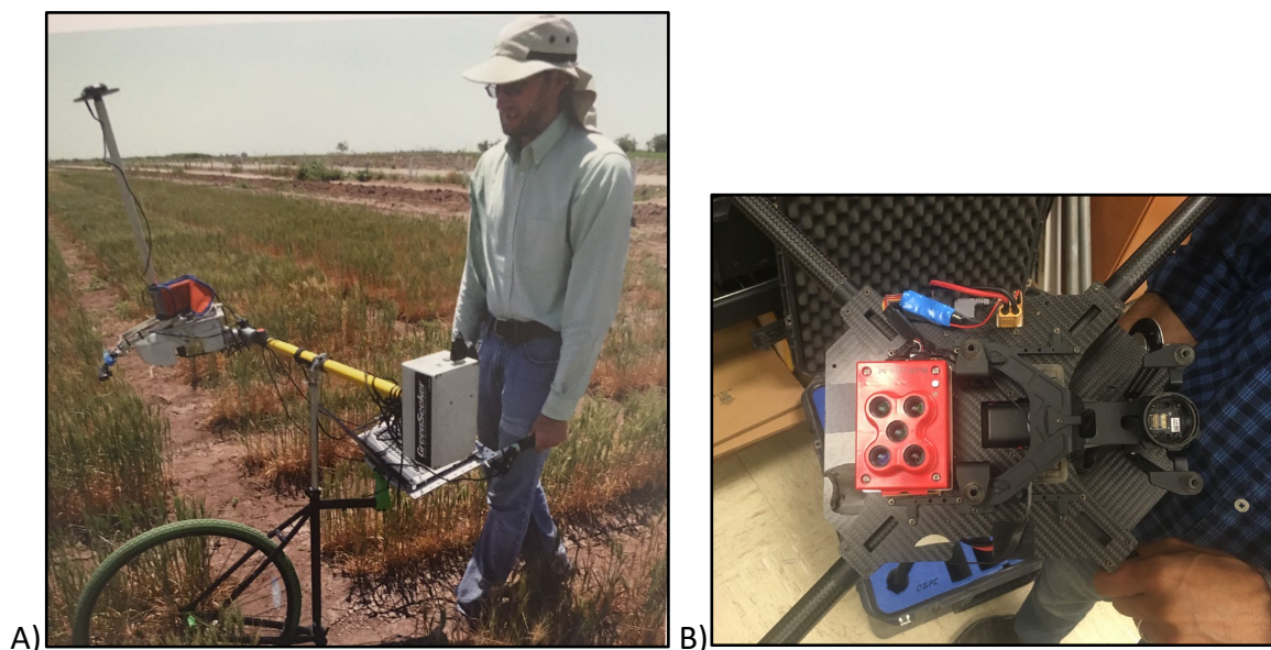
Figure 31. A) PhenoCart platform with NDVI, canopy temperature and georeferenced data at Obregon, Mexico. The platform integrates several commercial sensors, including GreenSeeker for spectral reflectance, an infrared thermometer, and a global navigation satellite system receiver (Source: Author, 2018) B) MicaSense RedEdge M optical sensor on UAV used at Kansas State University Wheat Breeding Program (Source: Author, 2018).
