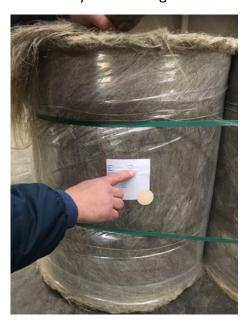
Figure 12: A 100kg bale of long line flax showing the traceability (origins) and exact weight in Belgium at Albert Brille's scutching mill
