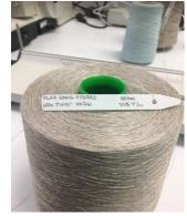
Figure 4: The finest Safilin yarn 50 Tex 245 T/m
