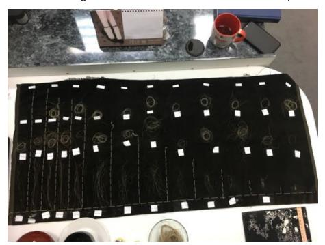
Figure 9: Determination of flax fibre lengths in the lab at the Institute of Natural Fibre and Medical Plants (<a href="https://iwnirz.pl/">https://iwnirz.pl/</a>)
