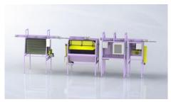
Figure 11: TapRoot Fibre Small Scale Scutching Mill
