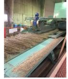
Figure 6: Breaking Machine
