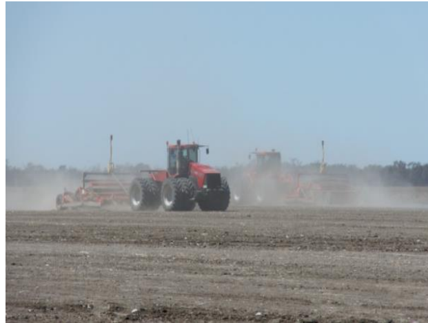
Figure 10 Equipment moving soils to level a field for irrigation. Photo Tony Balkwill
